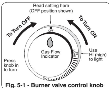
Fig. 5-1 - Burner valve control knob
